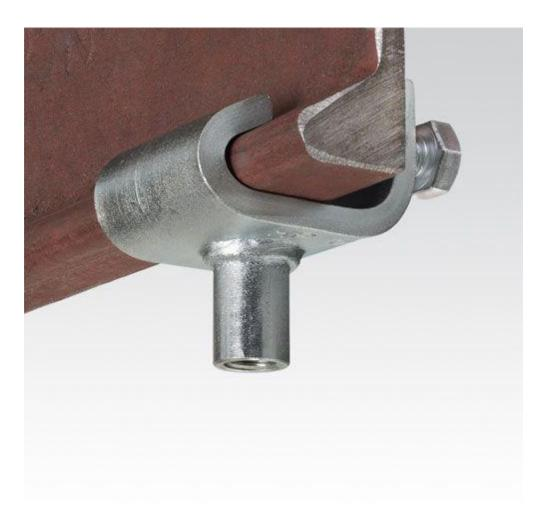
The HP-Clamp is the high-speed solution for simple mounting to holland profiles on ship structure without welding. It is suitable for direct, flexible mounting of metric M8/M10 threads to any desired position on the bulb profile and can be combined with MPC-Support channels for multiple pipe support systems.
